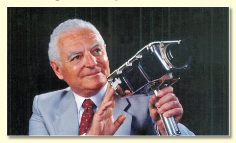
To bring us live television from the Moon, a team of Westinghouse engineers worked for 5 years to reduce a 180kg studio camera down to a 3kg handheld camera that could operate in the extreme conditions on the lunar surface.
